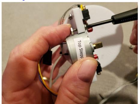
(7) Fit the second screw and nut to secure the other side of the stepper motor. Note that the stepper motor is mounted on the same side as the limit switches.
