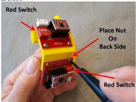
(10)The camera base with both driver boards should appear as shown. The left board controls the bottom stepper motor, and the right board controls the top stepper motor.
