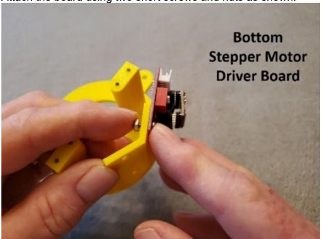
(9) Hold the camera base and driver board with the red switch block facing as shown. Hold the nut in place with your finger on the screw holding the assembly in place. Carefully place a nut on the screw turning the screw in a clockwise. Install the second screw. Gently tighten both screws to complete the assembly. Attach the second stepper driver board using two short screws as shown.
