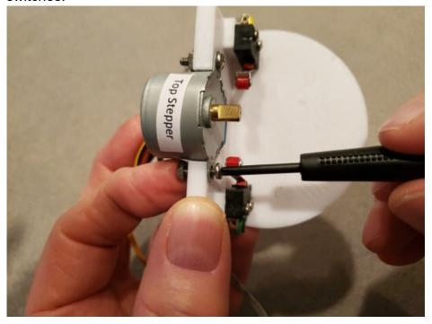
(8) There are two stepper motor driver boards that are mounted on the camera base. Position the driver board with the red switch block in the UP position. Attach the board using two short screws and nuts as shown.
