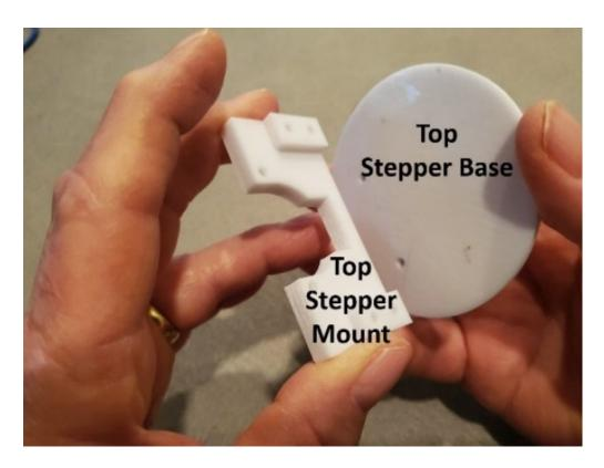
(3) When the top stepper mount and stepper based are assembled correctly the limit switch "pads" will appear as shown.
