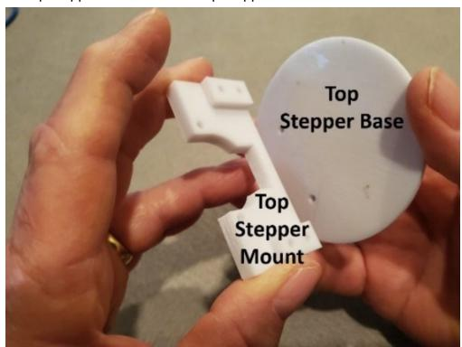
(2) Insert one of the self-tapping sheet metal screws through the bottom of the top stepper base. Don't fully tighten the first screw. Adjust the two parts so the second self-tapping sheet metal screw can be inserted through the top stepper base. Gently tighten both of the screws so that the two parts are stable. Over-tightening may damage the top stepper mount.
